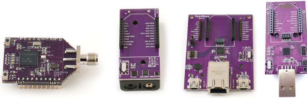
**Figure 2.1:** *OpenMote hardware ecosystem. From left to right: OpenMote-CC2538, OpenBattery, OpenBase, OpenUSB*
